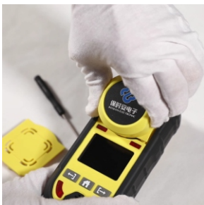
3.Align the pump with the bayonet on the machine and insert it.
