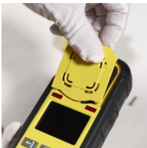
2.Remove the front natural diffusion card.
