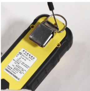
1.Unscrew the screw above the back clamp.
