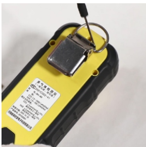
4.Tighten the connecting screws above the back clip.
